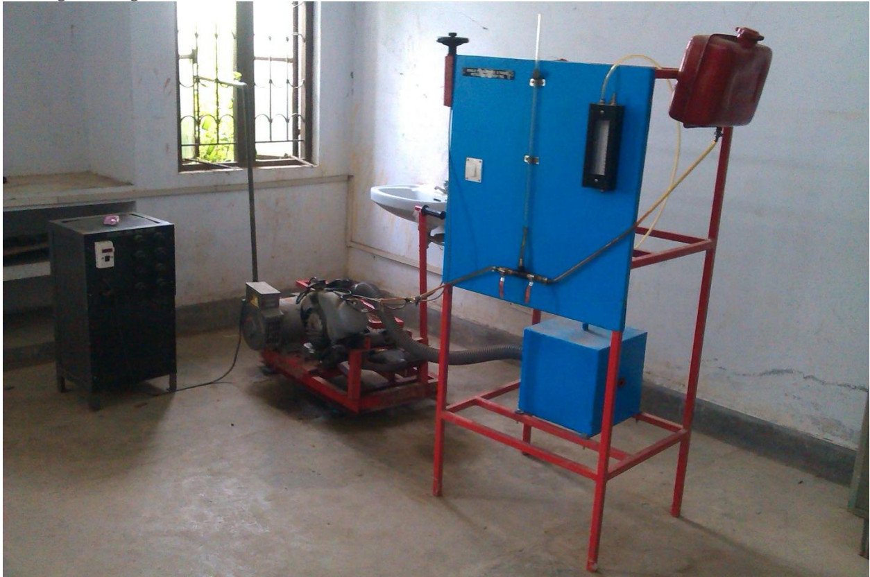
Figure:1 Experimental setup for the effect of methanol –gasoline blends
